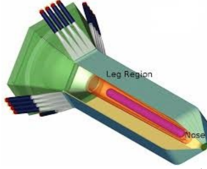
Figure 12: CLAS target and start counter (ST) diagram.
