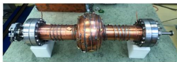
Figure 2. Left: Mock-up 1.3 GHz Cu cavity with the soldered capillary tube (inner diameter 2 mm, length 8 m). Right: Distribution of each temperature sensor on the cavity.
