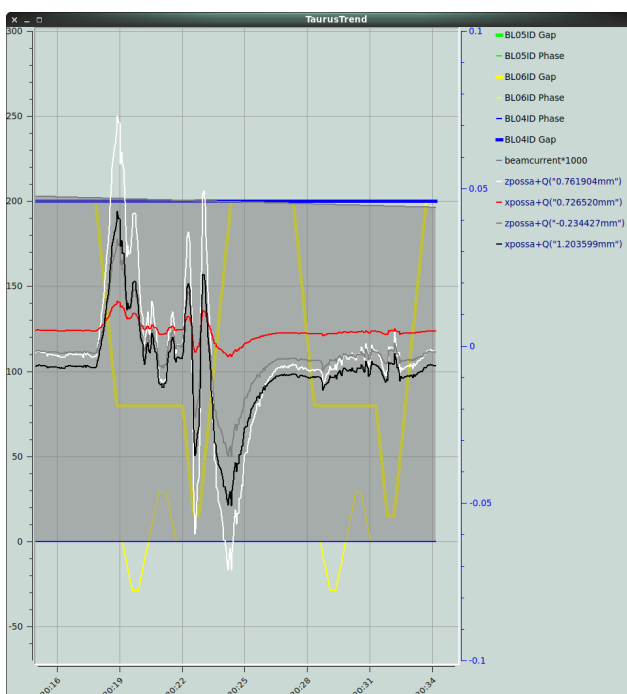
Figure 2: Effect of PHELIX undulator movement without and with correction.
