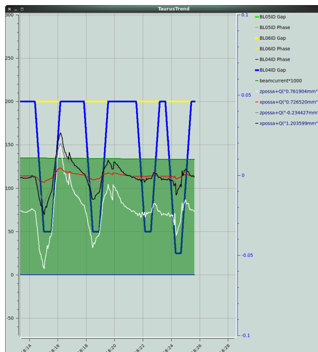
Figure 3: Test of new power supplies for the DEMETER undulator.
