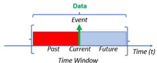
Figure 4: High speed data capture scheme with masking and event-based time window
