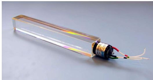
Figure 4.6: A \text{PbWO}_4 ECAL crystal with a vacuum phototriodes at the end [105].
