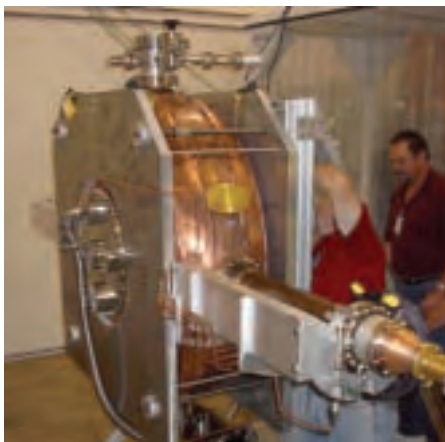
Muon Collider R&D RF cavity being prepared for tests at Fermilab. Credit: Yagmur Torun
