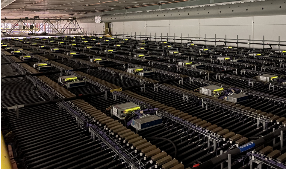
Figure 2.11: View from the top of the far detector, showing FEBs connecting to DCMs (grey boxes with yellow lights in the middle).
