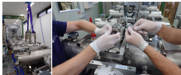
Figure 3: Tuner frame installation (left), tuning screw assembly (right).
