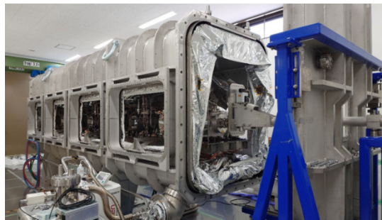
Figure 6: Main door closing with support of the CWT.
