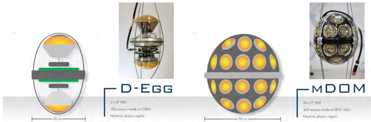
FIGURE 5.9 – New types of optical modules introduced in the IceCube-Upgrade: D-Eggs with 2 PMTs (left) and mDOMs with 24 PMTs (right). Figure courtesy of the IceCube Collaboration.
