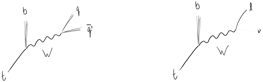
(a) Top quark decay with a hadronically decaying W boson. (b) Top quark decay with a leptonically decaying W boson.
