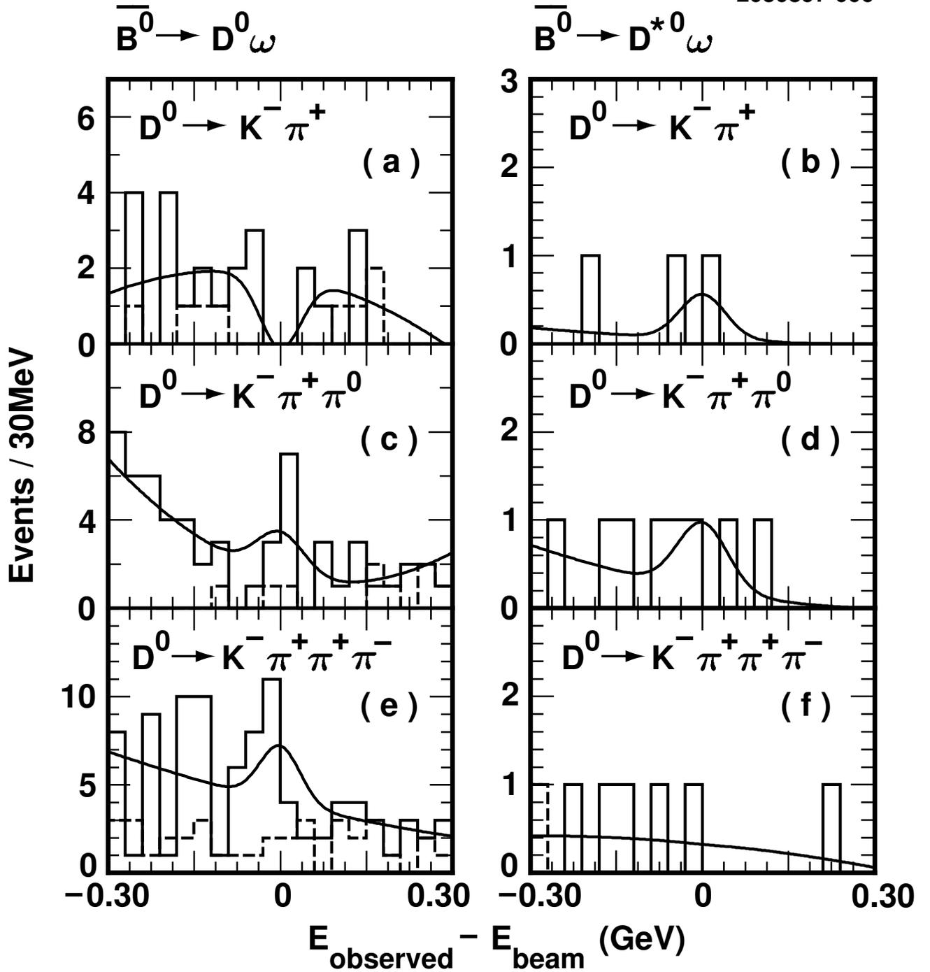
Figure 6:  $\Delta E$  distributions of  $\bar{B}^0 \rightarrow D^0 \omega$  and  $\bar{B}^0 \rightarrow D^{*0} \omega$  decay modes. Solid histograms are the  $\Delta E$  distributions of the 3.1  $\text{fb}^{-1}$  of data collected on the  $\Upsilon(4S)$  resonance, which are fit using background and signal functions. Dashed histograms are from the 1.6  $\text{fb}^{-1}$  continuum data sample.
