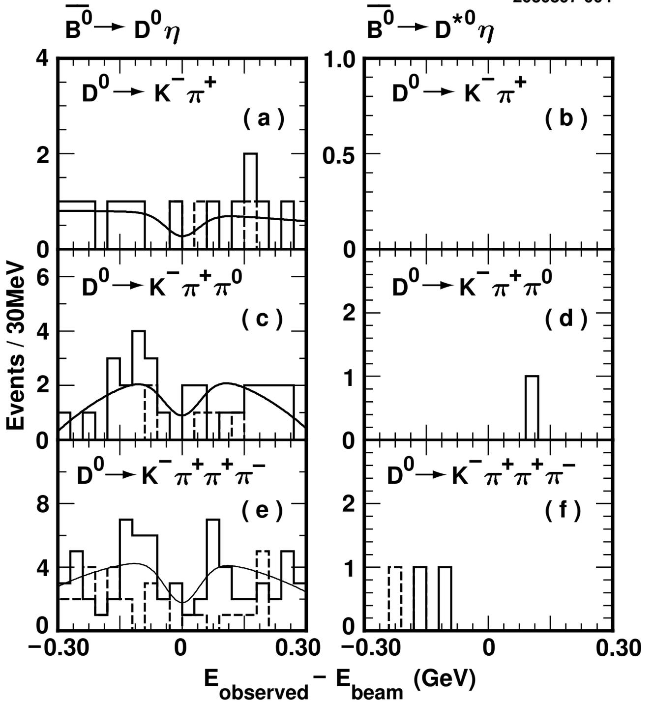
Figure 4:  $\Delta E$  distributions of  $\bar{B}^0 \rightarrow D^0 \eta$  and  $\bar{B}^0 \rightarrow D^{*0} \eta$  decay modes. Solid histograms are the  $\Delta E$  distributions of the 3.1  $\text{fb}^{-1}$  of data collected on the  $\Upsilon(4S)$  resonance, which are fit using background and signal functions. Dashed histograms are from the 1.6  $\text{fb}^{-1}$  continuum data sample.
