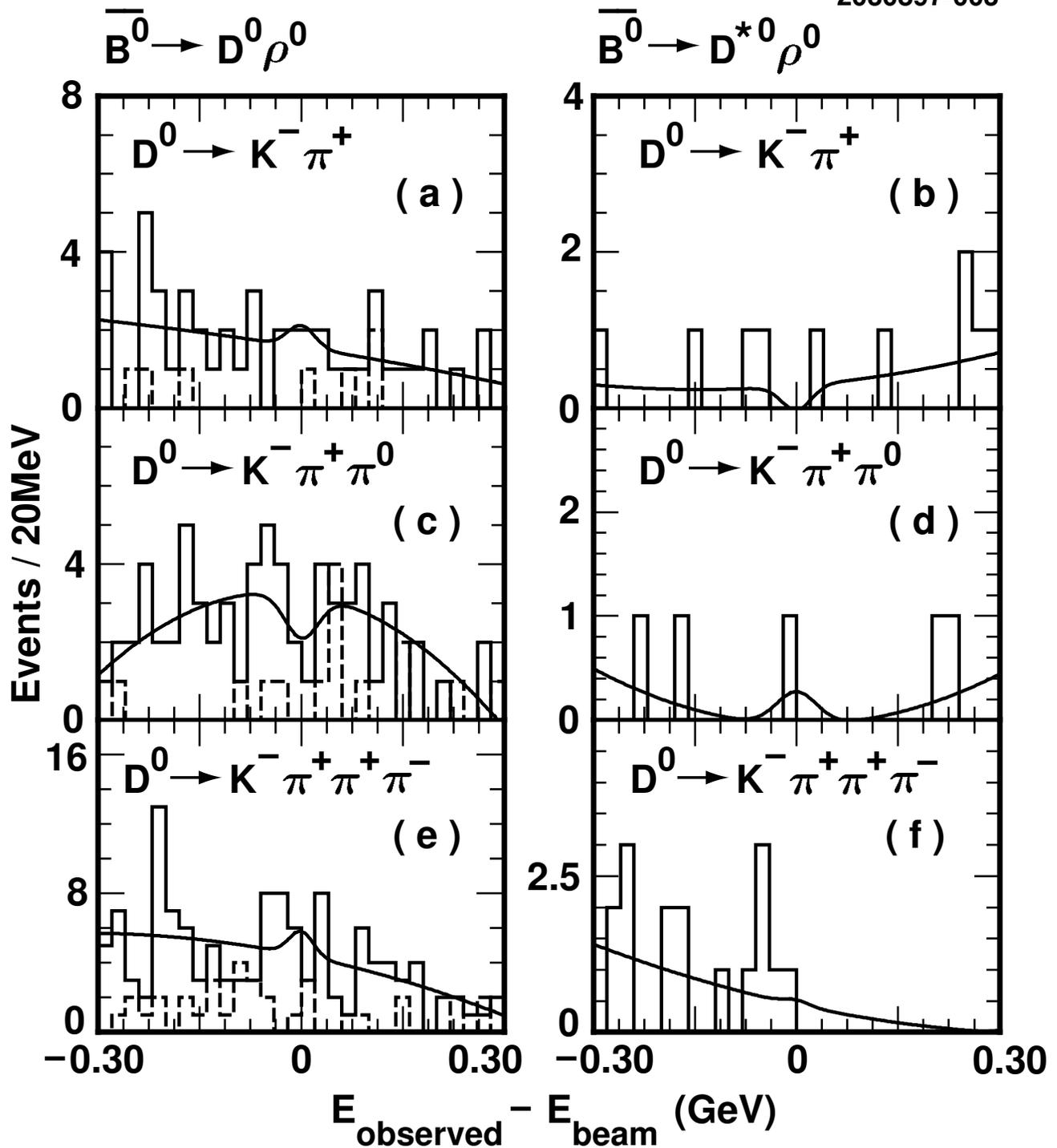
Figure 3:  $\Delta E$  distributions of  $\bar{B}^0 \rightarrow D^0 \rho^0$  and  $\bar{B}^0 \rightarrow D^{*0} \rho^0$  decay modes. Solid histograms are the  $\Delta E$  distributions of the  $3.1 \text{ fb}^{-1}$  of data collected on the  $\Upsilon(4S)$  resonance, which are fit using background and signal functions. Dashed histograms are from the  $1.6 \text{ fb}^{-1}$  continuum data sample.
