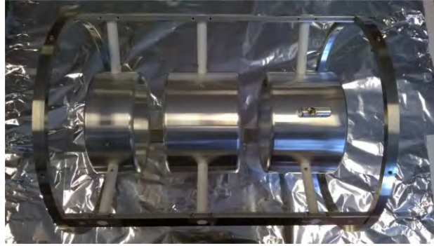
Figure 5.2 Triplet of pre-decelerating electrodes mounted on the aluminum frame with Macor rods.
