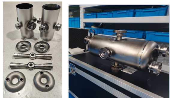
Figure 4: HWR1 prototype before and after welding.
