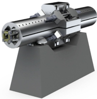
Figure 2: View of the compact APPLE-X undulator.
