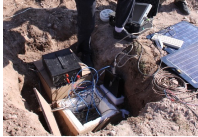
Figure 4: Installation of seismometer.
