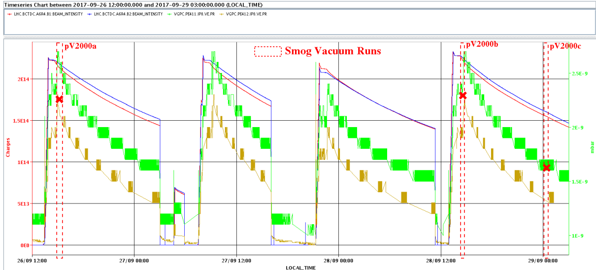
Figure 6: Time evolution of the gas pressure of the beam vacuum in the VELO area, measured by two Penning gauges (green and brown lines) during four LHC fills at nominal beam intensity in 2017. The intensity of the LHC beams is shown by the red (beam1) and blue (beam2) lines. The red crosses show, on arbitrary scale, the rate of beam-gas collisions, normalized to beam1 intensity, measured in three SMOG vacuum runs acquired during these fills. Note that the calibration scale of the gauges has large uncertainty, but the relative changes are significant, and in reasonable agreement with the beam-gas rate measurements.
