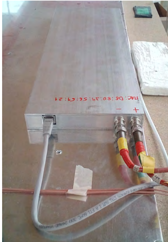
Figure 2.13: Photograph of the custom made HV power supply of the Tragaldabas detector. A voltage of \pm 5600 V is fed to each RPC plane, and it can be controlled with a web interface.
