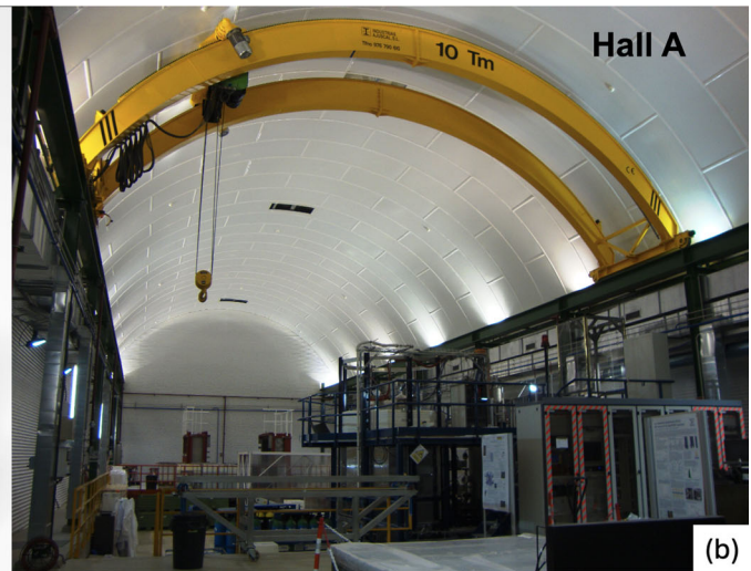
Fig. 62 a Cyclotron vault showing a bridge crane. Once the cyclotron is assembled, the bridge crane will be dismantled, and reconfigured for installation in the target hall. b Possible reconfiguration of the crane to adapt to the domed ceiling, photo is the crane in the Canfranc Laboratory hall in the Spanish Pyrenees [47]
