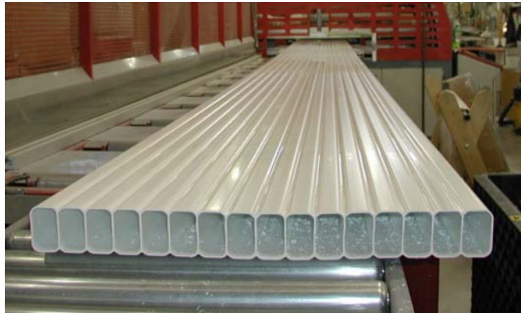
Figure 3.9: Structure of \text{NO}\nu\text{A} cells. The left shows the detection in one unit of \text{NO}\nu\text{A} detector. The right is the picture of one PVC extrusion module.
