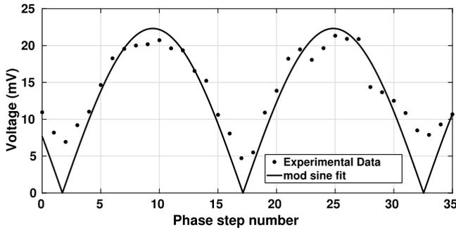
**FIGURE 11.** Peak-to-peak voltage monitored at the interferometer output versus RF phase difference between points A and B of experimental setup.
