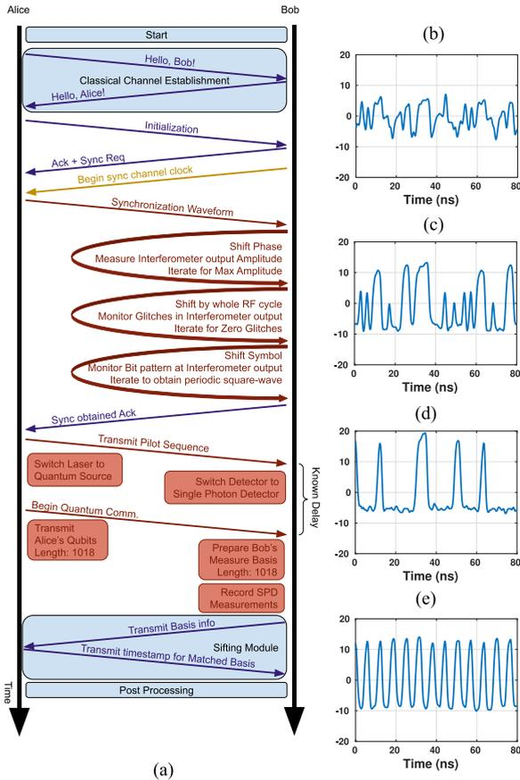
**FIGURE 10. Workflow stack of Software defined FC-QKD. On the left-hand side is (a) lattice diagram showing the signaling between Alice and Bob on the three channels—blue: Classical channel (Ethernet), yellow: S-channel, and red: Q-channel. On the right-hand side are the DSO outputs at various stages of the synchronization. (a) Before synchronization, (b) phase matched, (c) symbol boundaries aligned, and (d) frame synchronized.**
