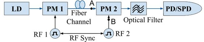
**FIGURE 1. Conceptual block diagram of FC-QKD system. Laser diode (LD), optical phase modulator (PM), photodetector (PD), and single-photon detector (SPD).**
