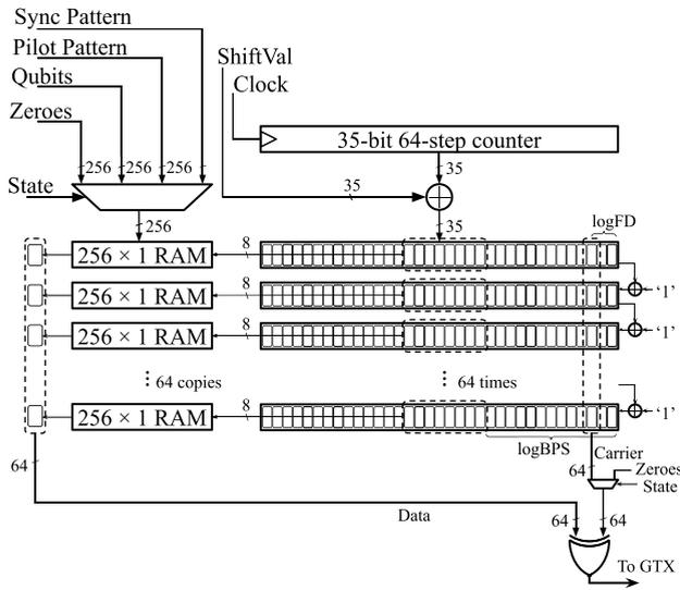
**FIGURE 6. Waveform generator module implemented on Xilinx Kintex-7 FPGA for generating square RF BPSK modulation.**
