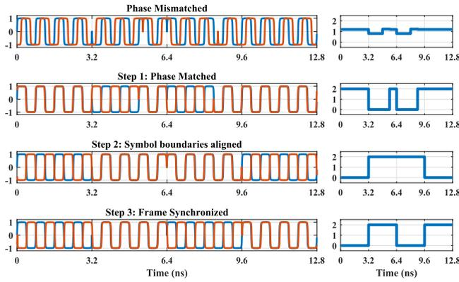
**FIGURE 4.** Steps in the proposed synchronization procedure. Optical phase at point A (blue) and electrical input to PM2 at point B (red). Waveforms in the right-hand side show the expected output from the photodetector at each step of the workflow.
