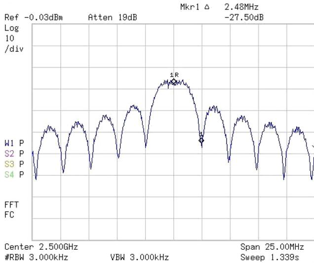
**FIGURE 7.** Measured spectrum of RF BPSK modulated signal generated by waveform generator module shown in Fig. 6. A  $2^9$ -length PRBS was used as modulation data.
