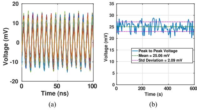
**FIGURE 13.** Plots to demonstrate interferometer stability. (a) Output of DSO synchronization signature monitored every 5 s for 10 min. (b) Peak-to-peak voltage of the synchronization signature with respect to time.
