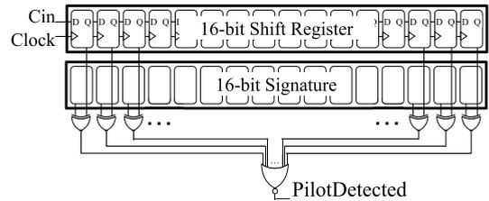
**FIGURE 9.** Pilot detector module implemented on Bob’s FPGA.
