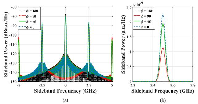
**FIGURE 3.** (a) Plot of PSD at the output of PM2 showing sideband interference. (b) Zoomed PSD of first sideband for phase differences of 0°, 45°, 90°, and 180°. Note that y-scale of (a) is in decibels, and y-scale of (b) is linear.
