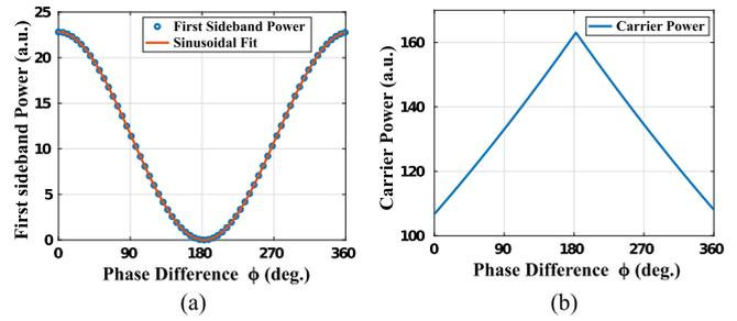
**FIGURE 2.** Plot of power of first sidebands  $\omega_0 \pm \Omega$ , and carrier  $\omega_0$  as function of phase difference  $\phi$  between the RF signals generated by Alice and Bob.
