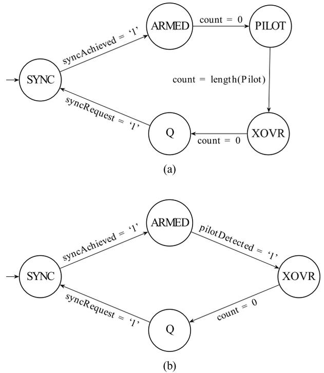
**FIGURE 8.** State diagram representation of the FSM modules implemented on the FPGAs at (a) Alice and (b) Bob.
