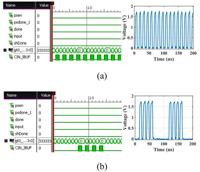
**FIGURE 12.** (a) Synchronization signature and (b) quantum transmission interference detected on Bob’s FPGA and DSO (inset) when a qubit sequence of  $0 \times 8461\dots$  and  $0 \times 2E9E\dots$  was sent by Alice and Bob, respectively.
