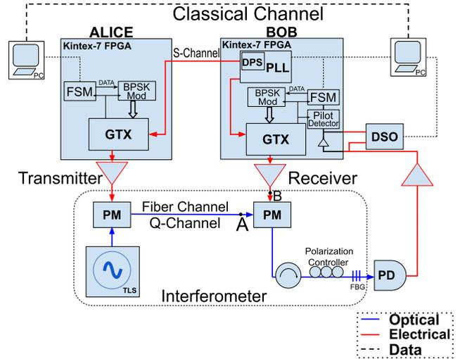
**FIGURE 5.** Experimental setup. Tunable laser source (TLS), phase modulator (PM), fiber Bragg grating (FBG), photodiode (PD), phase-locked loop (PLL), gigabit transceiver (GTX), dynamic phase shifter (DPS), finite-state machine (FSM), and digital storage oscilloscope (DSO).
