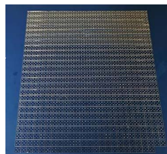
Figure 3. 623 14 x 14 x 1.5 mm LYSO plates for a LYSO/W Shashlik matrix
