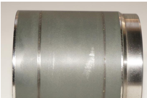
Figure 7: Ceramic Coated Sleeve (52 mm length, 50 mm diameter, 0.5 mm ceramic coating) shows oil residues but no signs of roping after 9000 operating hours.
