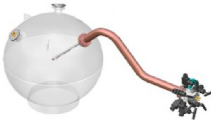
Figure 3.7: SEDINE. The S-shaped tube connects the sphere with the outside of its shielding [30].
