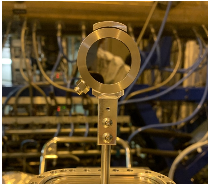
Figure 2.25. Picture of a large aperture silicon detector (Type 3) before installation inside a diagnostic box.
