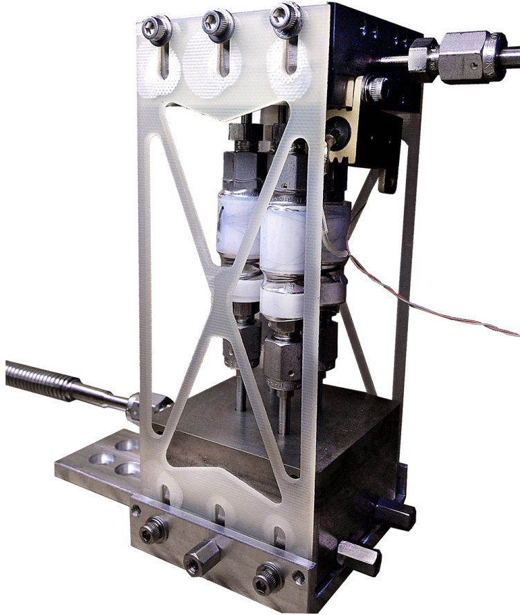
Figure 2.14: The capillary assembly installed prior to Run 10. Four capillaries connect the 4 K main tank box (bottom) to the 1.8 K superfluid box (top). The double volume structure is supported by two 1/32 inch thick G-10 flexures. The thermal load conducted through these flexures is negligible compared to the cooling power from the superfluid helium. Porous stainless steel Mott filters located below each capillary prevent ice and other dirt from entering and clogging this high impedance tubing. Superfluid helium exits the capillaries in the smaller of the two boxes (top) which is connected to the superfluid tank through 6 inch long bellows tubing with a 1/8 inch diameter.
