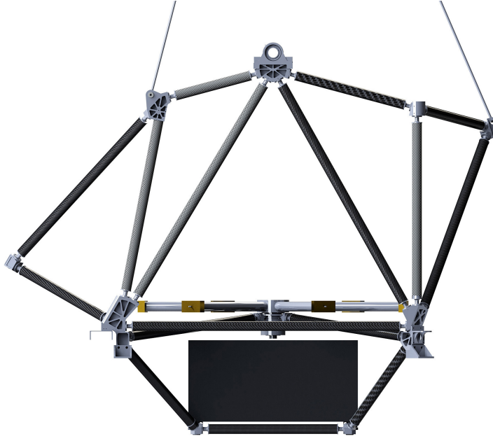
Figure 2.31: A rendering of the gondola assembly without the flight cryostat. The reaction wheel is mounted over the enclosure for the CSBF support instrumentation package. The trunnions of the flight cryostat are mounted to the pillow block shown at the top of the figure.
