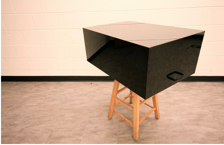
Figure 2.30: The covered FTS sitting on a lab stool. The mass of the entire assembly is 23 kg, making it possible to transport by a single person.
