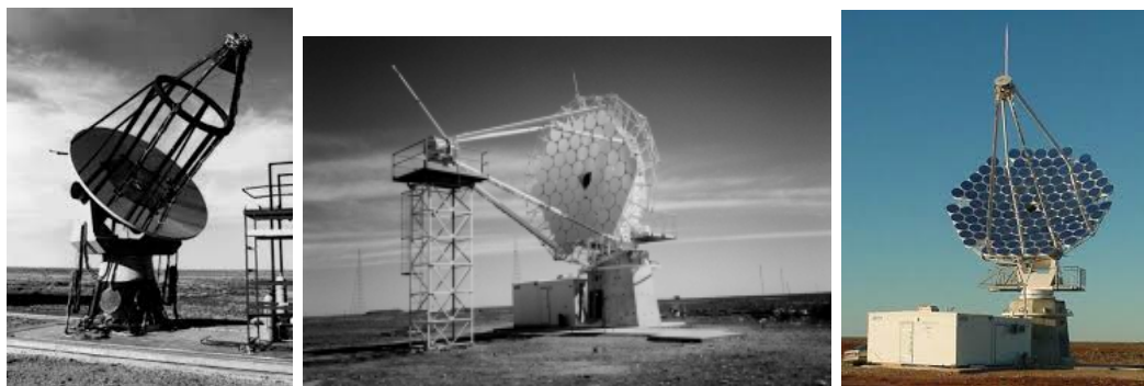
Figure 1.30: Evolution of the CANGAROO project throughout the years. On the left, the 3.8-m CANGAROO-I telescope, in the central image the CANGAROO-II 7-m telescope, and on the right image one of the 10-m telescopes from the CANGAROO-III array. Image credits: CANGAROO Collaboration (2000) and Mori (2003).
