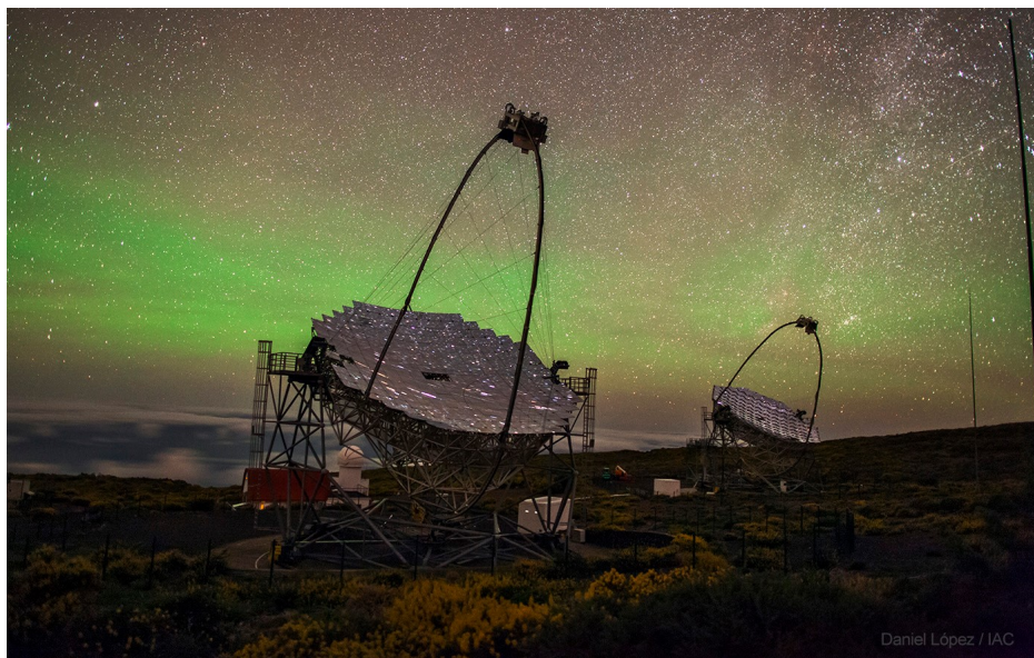
Figure 1.34: The 17 m diameter MAGIC telescopes located at Roque de los Muchachos, La Palma. MAGIC is optimised to perform gamma-ray observations from 50 GeV and up to 50 TeV, and to follow fast transient phenomena with its rapid repositioning system. Image credit: Daniel Lopez; https://magic.mpp.mpg.de/ , last accessed on 01/08/22.
