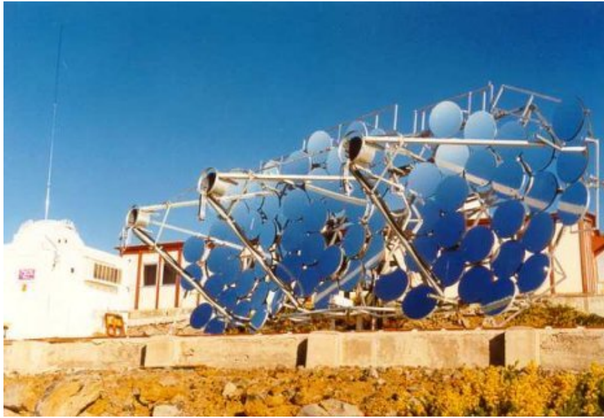
Figure 1.27: Mark IV telescope at La Palma, Canary islands, Spain. The Mark IV was a portable telescope designed for short observing campaigns, it was operated in La Palma during June-October 1988. Image credit: Durham University, Gamma-ray Group, https://www.dur.ac.uk/cfai/vhegammaraygroup/grouphistory/australia/ , last accessed on 01/08/22.
