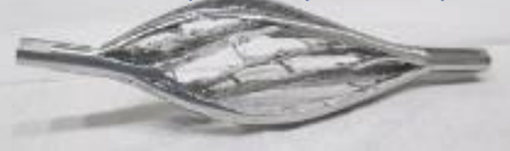
Metal rod exploded by beam impact
