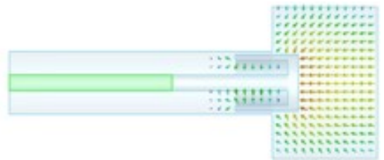
Figure 2: Electric Field profile simulated with a partially inserted plunger, Credits: Dr. Cervantes, SQMS
