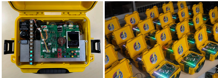
Figure 2: (left) Photo of a compact gamma-ray monitor (CoGaMo) used by the citizen science "Thundercloud Project." (right) Multiple Cogamos with turning on the LED lights on the detector boxes.
