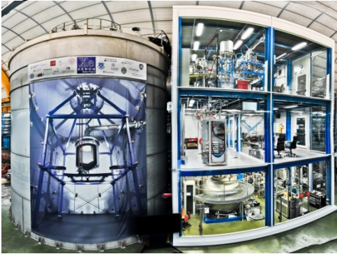
Caption: A cut-out view of the XENON1T experiment in the Gran Sasso National Laboratory. The 2-ton liquid xenon target hangs in the middle of the large water tank on the left. Auxiliary systems are located in the three-story building on the right. Credit: Roberto Corrieri and Patrick De Perio.
