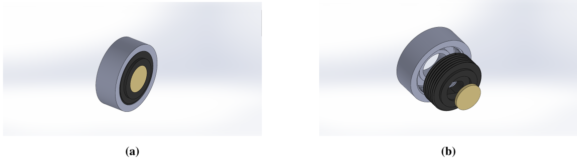
Figure 10: Solidworks images of the assembled (left) and exploded (right) housing of the acoustic receiver. The threading will allow for the capsule to be screwed into the exterior and apply pressure to the PCB keeping it in place. No PCB has been fit into the assembly in this drawing, but there is a cavity where it will be inserted. The gold part is the piezoelectric disk with a 20 cm diameter.
