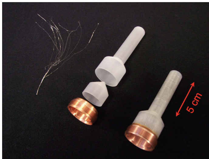
Figure 2.17: A typical target cell (left) and individual components separated (right). Image was taken from [27]
