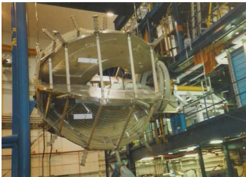
Figure 2.12: Photograph of the CLAS toroidal magnet. Image was taken from [34].
