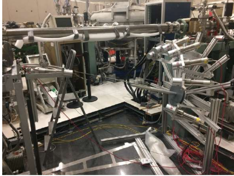
Figure 5.3: Experimental setup used at LNS to calibrate the ReD neutron spectrometer. Eight of the nine liquid scintillator detectors were placed on the supporting structure (far detectors), while the ninth (near detector) faced a ^{252}\text{Cf} neutron fission source in order to tag fission events (details in the text).
