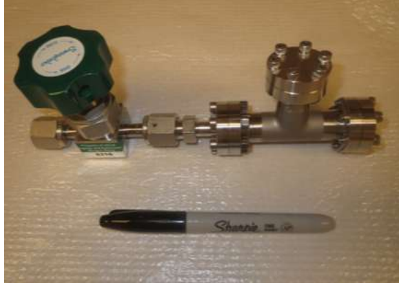
Figure 4.1: Photo of the ^{83}\text{Rb} trap deployed in the recirculation loop of ReD used for the calibration measurements with the ^{83\text{m}}\text{Kr} \gamma -rays source.
