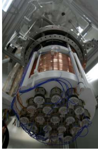
Figure 2.3: A picture of the DarkSide-50 LAr TPC from the bottom point of view. The array of 19 3-inch bottom PMTs is also visible.
