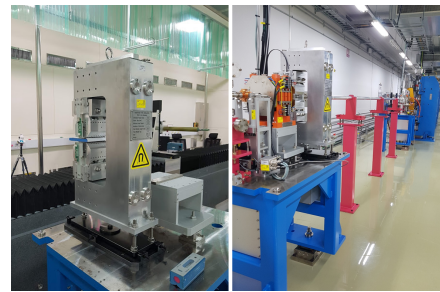
Figure 4: RTU in field measurement bench (left) and installation in front of hard X-ray undulator beamline (right).
