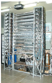
Figure 5. Stack of twelve 1\text{ m}^2 glass RPC at TIFR.
