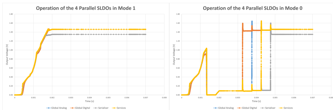
Figure 5. Functional simulation of 4 SLDO AncASIC in Modes 0 (all outputs enabled at startup) and 1 (all outputs disabled at startup and manually enabled). The 4 supplies represent those of the EIC-LAS.
