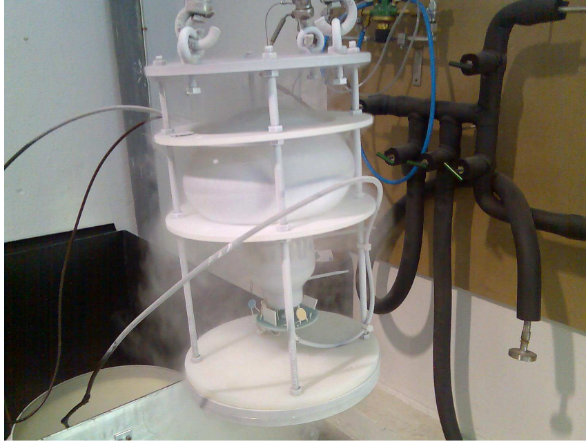
Figure 2.10: PMT inside the supporting structure after extraction from liquid argon bath.
