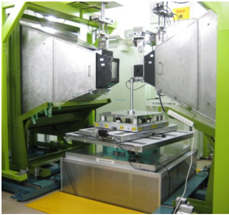
Figure 6: Neutron diffraction measurement facility at the BL-19 (TAKUMI) of J-PARC MLF.
