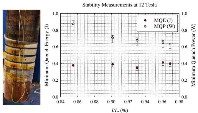
Fig. 6. Left: Picture of instrumented Nb<sub>3</sub>Sn Rutherford bifilar cable sample ID2. Right: Minimum quench energy and power obtained for the 40-strand Nb<sub>3</sub>Sn cable sample at 12 T and various transport currents (right) [10].
