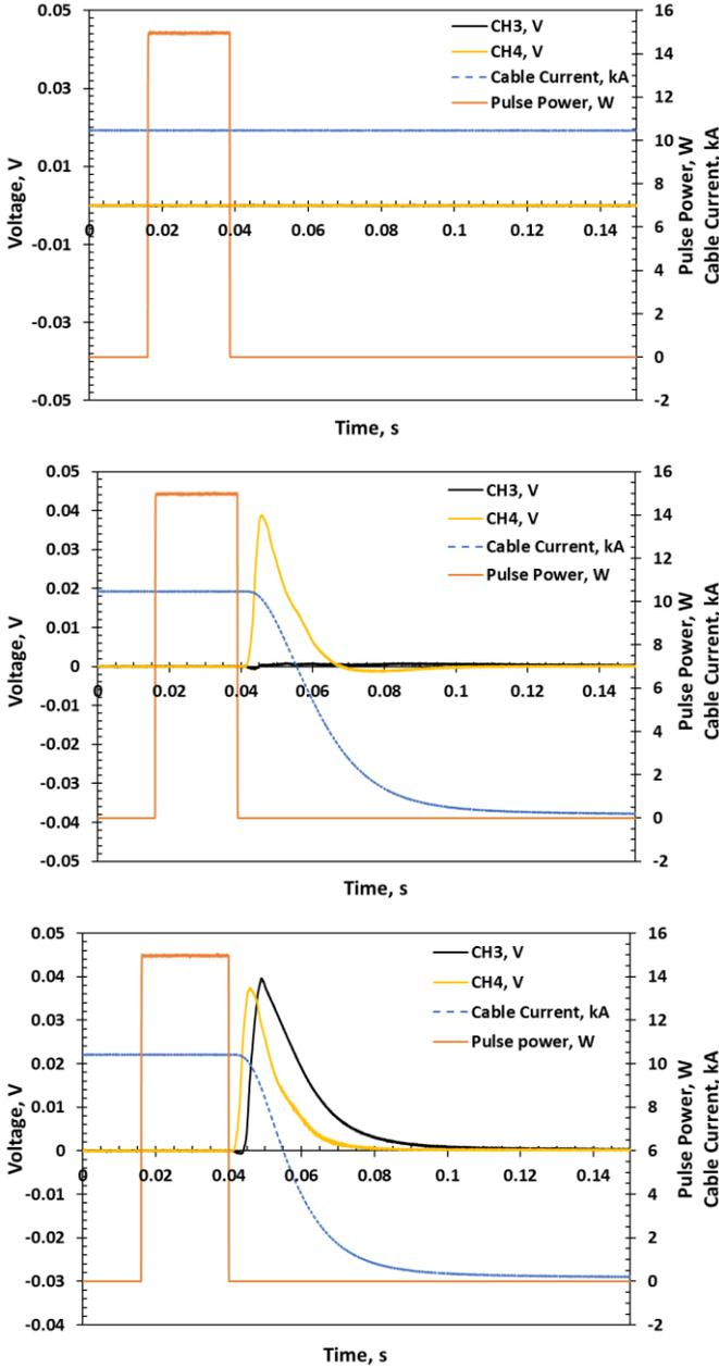
Fig. 11. Voltage signals obtained for channels CH3 and CH4 in the  $MQE$  test of the NbTi cable outfitted with the high- $C_p$  ribbons at 6 T and 47% of  $I_c$  (6T) for the cases of input pulse energy lower than the  $MQE$  value (top), at the  $MQE$  value (middle) and above the  $MQE$  value (bottom) of 0.34 J. In the top plot both channels signals are at zero. At constant pulse power of ~15 W, the cable  $MQE$  is determined by the pulse duration.
