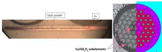
Fig. 1. Left: Cross section of Cu tape with  $\text{Gd}_2\text{O}_3$  inside, 30% of the cross section is  $\text{Gd}_2\text{O}_3$  (courtesy of Hypertech). Right: Hyper Tech Sn-in-Tube  $\text{Nb}_3\text{Sn}$  wire with 48 regular Nb-Sn subelements and 13 high- $C_p$  ones made of  $\text{Cu}/\text{Gd}_2\text{O}_3$  [6], [7].
