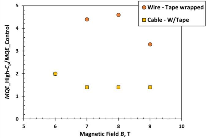
Fig. 19. Gain values of wire wrapped with high- $C_p$  ribbon and of cable outfitted with it as function of magnetic field for measurements performed at 90%  $I_c$ .
