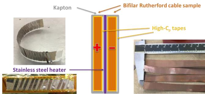
Fig. 8. Experimental schematic of SC bifilar cable sample.
