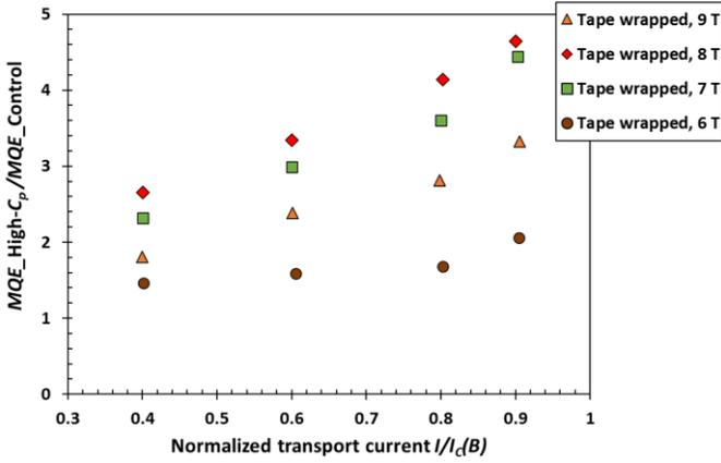
Fig. 14. Gain at various magnetic fields of wrapping the NbTi wire with the thin high- $C_p$  tape, or the  $MQE$  ratio between the  $MQE$  obtained with the ribbon and that without, as function of normalized transport current.
