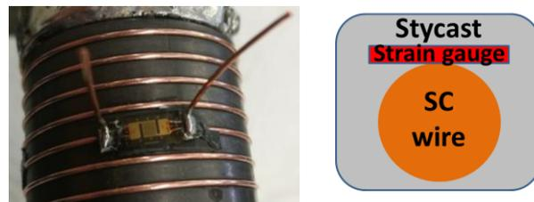
Fig. 2. Strain gauge used as heater mounted on wire (left) and experiment schematic, showing the strain gauge mounted on a SC wire (right).
