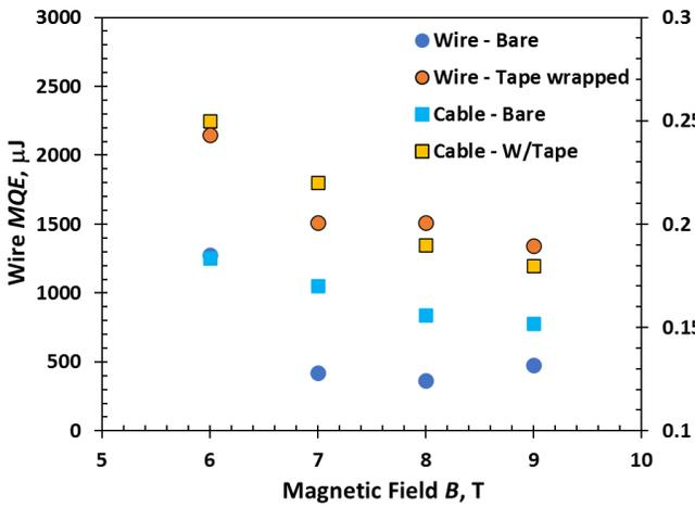
Fig. 17. Wire and cable  $MQE$  values as function of magnetic field for measurements performed at 80%  $I_c$ .
