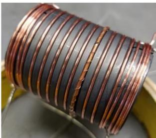
Fig. 3. NbTi superconducting wire sample wrapped with Hyper Tech high- $C_p$  tape cut down to  $\sim 1$  mm width, along half a turn of the specimen.
