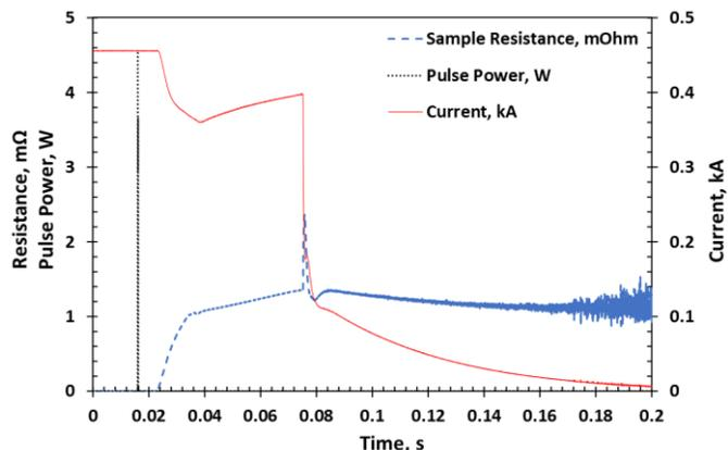
Fig. 5. Sample resistance, or more accurately sample voltage over current ratios obtained in the  $MQE$  test of the bare NbTi extracted wire at 6 T and 90% of  $I_c$  (6T). Pulse power and sample current are also shown.
