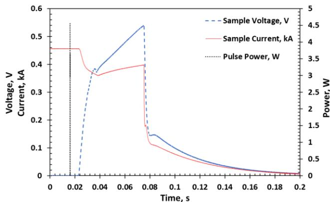
Fig. 4. Sample voltage signal obtained in the  $MQE$  test of the bare NbTi extracted wire at 6 T and 90% of  $I_c$  (6T) with input pulse energy at the  $MQE$  value. Pulse power and sample current are also shown.
