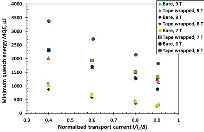
Fig. 13.  $MQE$  results at various magnetic fields for bare extracted NbTi wire and for NbTi wire sample wrapped with Hyper Tech high- $C_p$  ribbon as function of normalized transport current in the sample.
