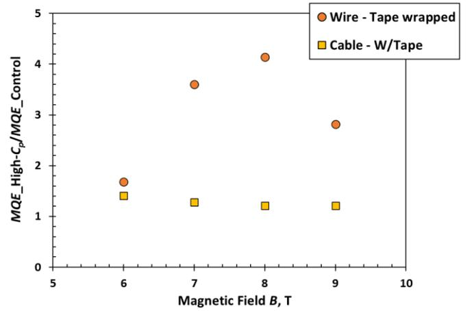
Fig. 18. Gain values of wire wrapped with high- $C_p$  ribbon and of cable outfitted with it as function of magnetic field for measurements performed at 80%  $I_c$ .
