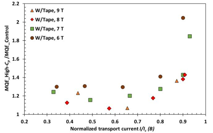
Fig. 16. Gain at various magnetic fields of outfitting a NbTi cable with high- $C_p$  tape, or the  $MQE$  ratio between the NbTi cable's  $MQE$  obtained with the ribbon and that without, as function of normalized transport current.
