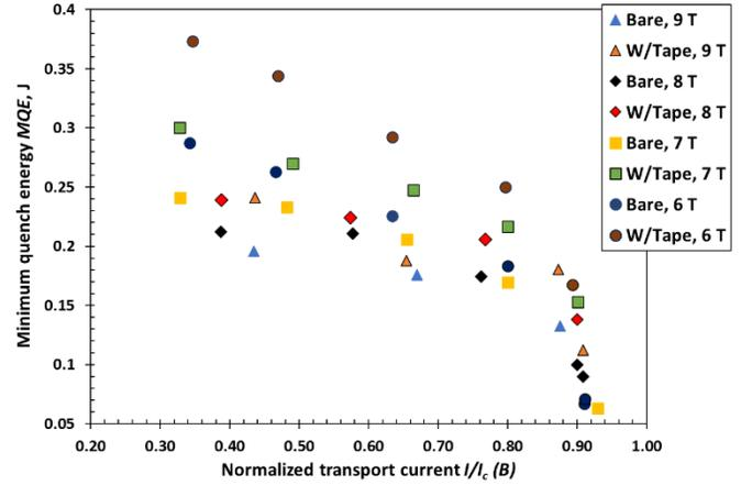
Fig. 15.  $MQE$  results at various magnetic fields for NbTi Rutherford cable sample ID1 as function of normalized transport current.
