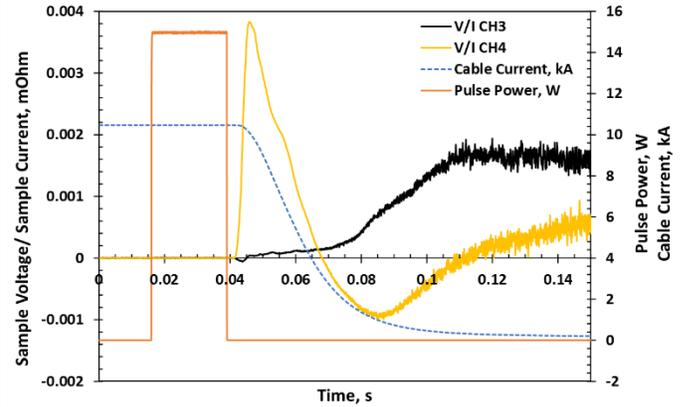
Fig. 12. Sample voltage over sample current ratios obtained for voltage tap channels in the  $MQE$  test of the NbTi cable at 6 T and 47% of  $I_c$  (6T).
