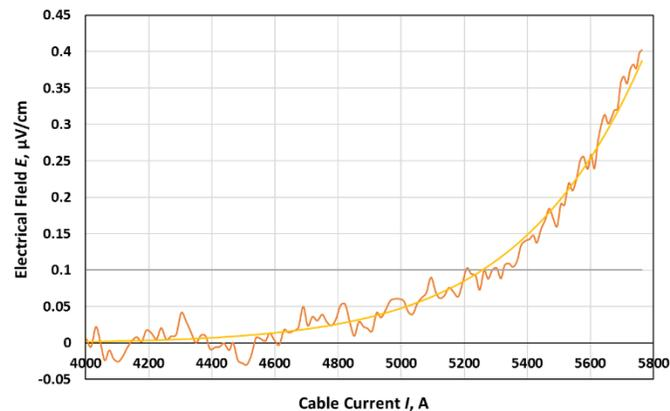
Fig. 9. NbTi cable's electrical field,  $E$ , vs. transport current,  $I$ , for cable test at 9 T. The  $I_c$  was determined using an electrical field criterion of  $0.1 \mu\text{V}/\text{cm}$ .
