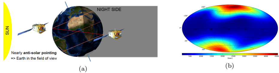
Fig. 8. SVOM pointing strategy. (a) Illustration of the anti-solar pointing that allows telescopes on the night side of the Earth to observe SVOM alerts promptly. (b) ECLAIRS one year exposure map in galactic coordinates.
