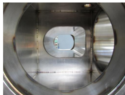
Figure 4: Inner cavity of BC special-shaped vacuum chamber.
