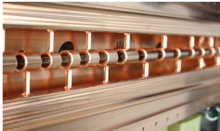
Figure 4. The fabricated center plate of the IH-DTL.
