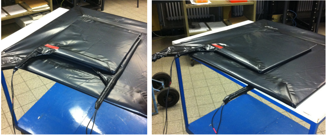
Figure 3.5: The setup used to measure the efficiency of the small (left) and large (right) muon detectors.
