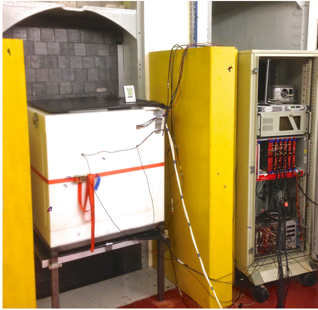
Figure 3.11: The NEMENIX detector with closed shielding and LB (top) and LR (bottom) muon planes.
