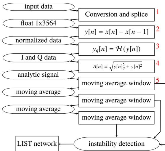
Figure 1: The LHC online instability detection pipeline.
