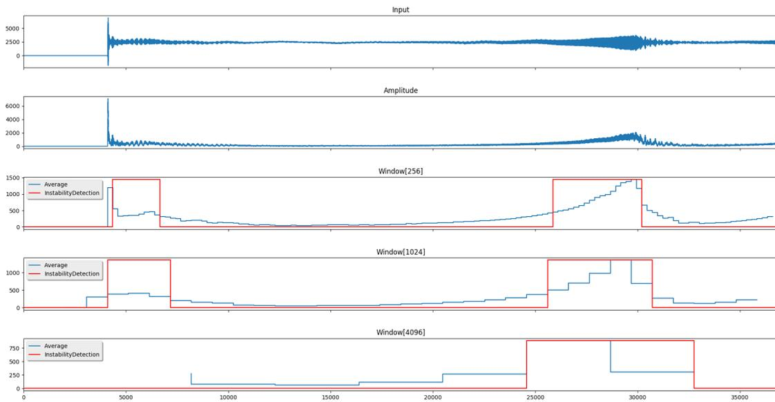
Figure 2: Output from instability detection with data from observations.
