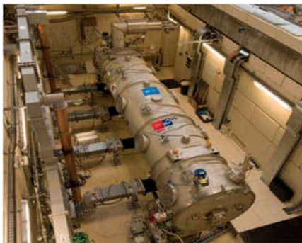
Figure 4: M-ECCTD in the CEA test stand.
