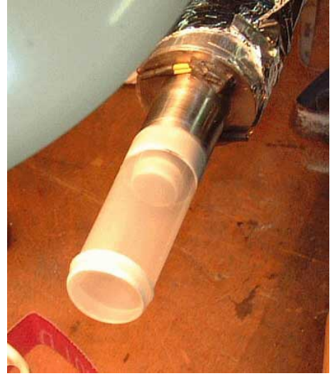
Figure 34: Picture of the Liquid-hydrogen target vessel. The entrance window is glued on a stainless-steel tube.
