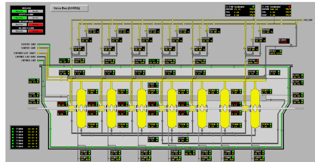
Figure 6: cryogenics control-system during tests.
