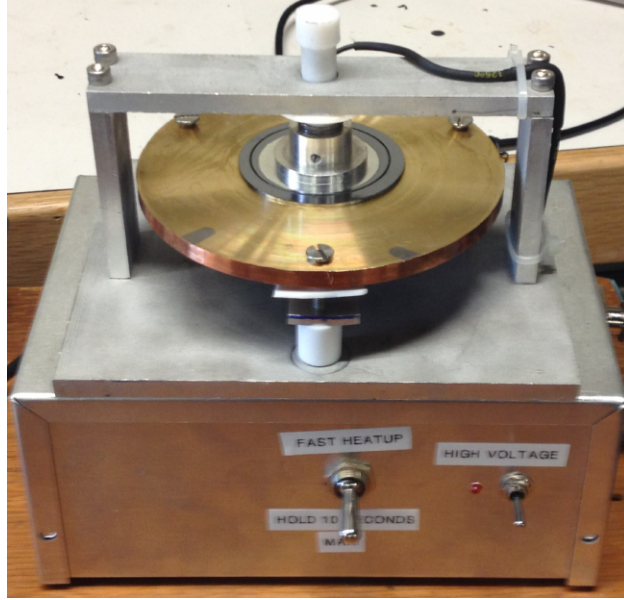
Figure 4.8: Custom Li drifting apparatus used to drift 2"-diameter prototype Si(Li) detectors.
