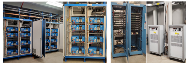
Figure 9: Unipolar power supplies (left) and bipolar supplies with bulk supplies (right) under test.
