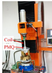
Figure 12: Rotating coil measurement.
